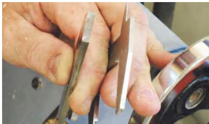
▲ Pic.6 Sizing cuts are generally made with a parting tool. Make sure the callipers are narrower than the tool
